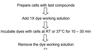
Analyze sample with a flow cytometer at Ex/Em = 542/556 nm
